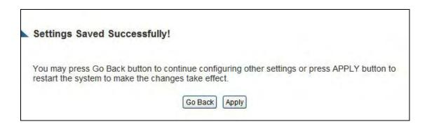
Press 'Go Back to save the settings made and go back to the web management interface; press 'Apply' to save the settings made and restart the Outdoor Wireless-N Smart Repeater so the settings will take effect after it reboots.
