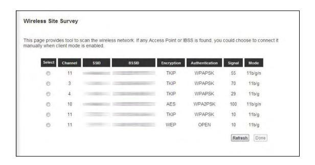
After you have selected a wireless Internet connection network, you may configure the security settings for that network if required. Select the security type and the encryption method and enter the appropriate key for the network you plan on connecting to.
