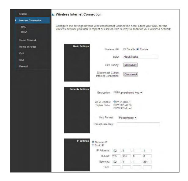
You may manually enter the SSID of the wireless network you plan on connecting to or you can click 'Site Survey' to have the web interface scan for local networks in your vicinity. (See Site Survey Menu below)
