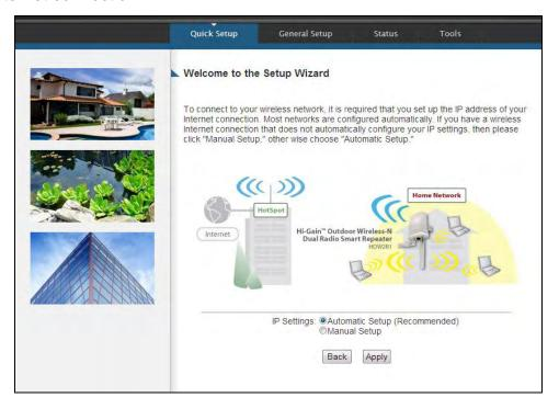
Select "Automatic Setup" to have the wizard automatically configure the IP settings of your Internet Connection. Most networks use Dynamic IP settings to automatically assign IP Addresses to incoming connections. If the network you are connecting does not use Dynamic IP settings you will need to manually configure (Manual Setup) your IP settings.
