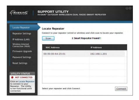
Note: before making any configurations on the Utility, you MUST be connected to a Repeater. The status of the Utility and Repeater connection is displayed on the bottom left corner.
