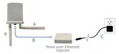
Set up your hardware according to the diagram above for the initial setup of the Outdoor Dual Radio Smart Repeater. After the initial setup is complete, you may mount the Outdoor Dual Radio Smart Repeater in your desired location.
