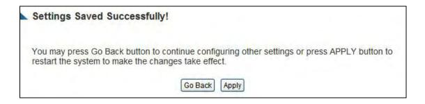
Press 'Go Back to save the settings made and go back to the web management interface; press 'Apply' to save the settings made and restart the Outdoor Wireless-N Smart Repeater so the settings will take effect after it reboots.
