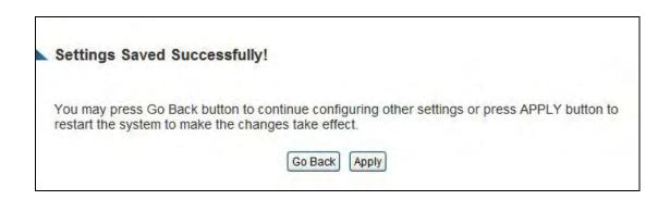
Press 'Go Back to save the settings made and go back to the web management interface; press 'Apply' to save the settings made and restart the Outdoor Wireless-N Smart Repeater so the settings will take effect after it reboots.
