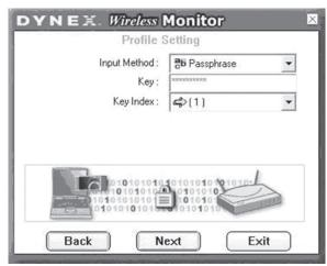
When encrypted information is received it is only accepted if it decrypts correctly. This happens only if the computer has the WEP Key used by the access point. This screen lets you enter the WEP key.
