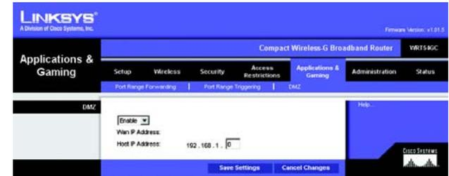
Figure 5-29: Applications and Gaming Tab - DMZ
