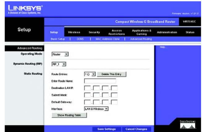
Figure 5-12: Setup Tab - Advanced Routing (Gateway)
