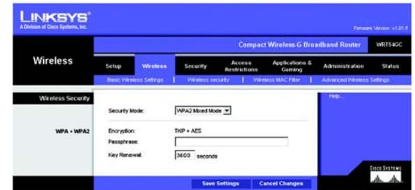
Figure 5-18: Wireless Tab - Wireless Security (WPA2 Mixed Mode)
