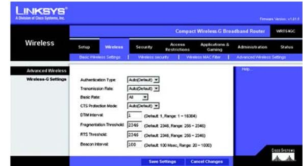
Figure 5-21: Wireless Tab - Advanced Wireless Settings
