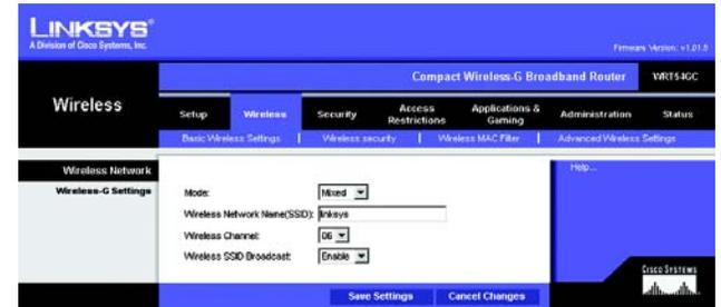
Figure 5-14: Wireless Tab - Basic Wireless Settings
