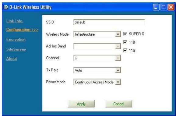
**SSID:** The Service Set Identifier is the name assigned to the wireless network. The factory SSID setting is **default**.
