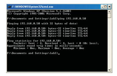
Go to **Start** > **Run** > type **cmd**. A window similar to this one will appear. Type **ping xxx.xxx.xxx**, where **xxx** is the **IP address** of the wireless router or access point. A good wireless connection will show four replies from the wireless router or access point, as shown.
