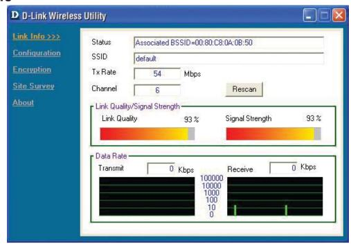
**Status:** Displays the MAC address of the access point or router to which the DWL-G650M is associated.
