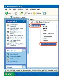
Assigning a Static IP Address in Windows XP/2000
