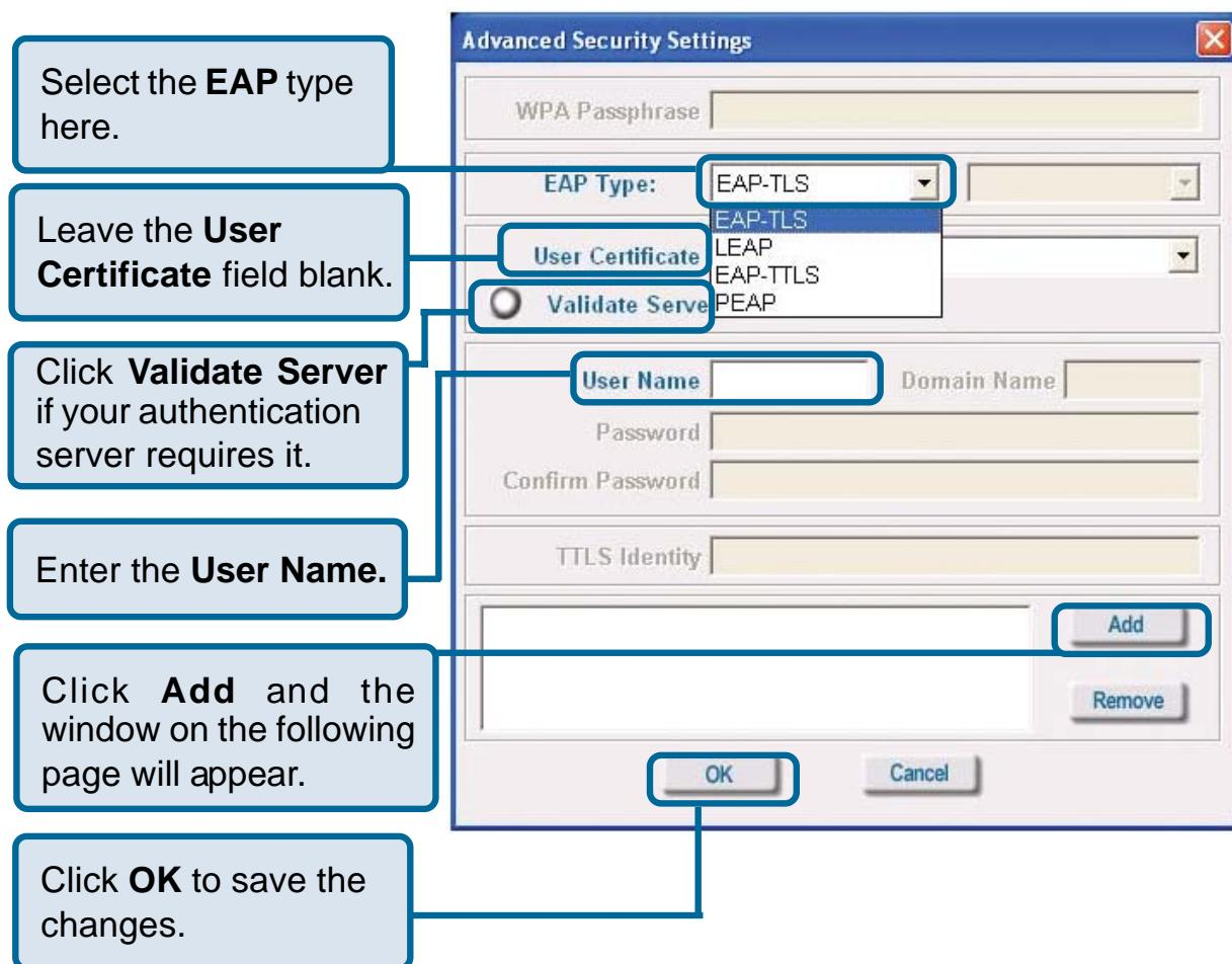
**EAP Type:** Extensible Authentication Protocols (EAP-TLS, LEAP, EAP-TTLS, PEAP) allow devices on the network to request authentication from the RADIUS server in the network. All the devices on the network must use the same EAP type when using a RADIUS server for authentication.
