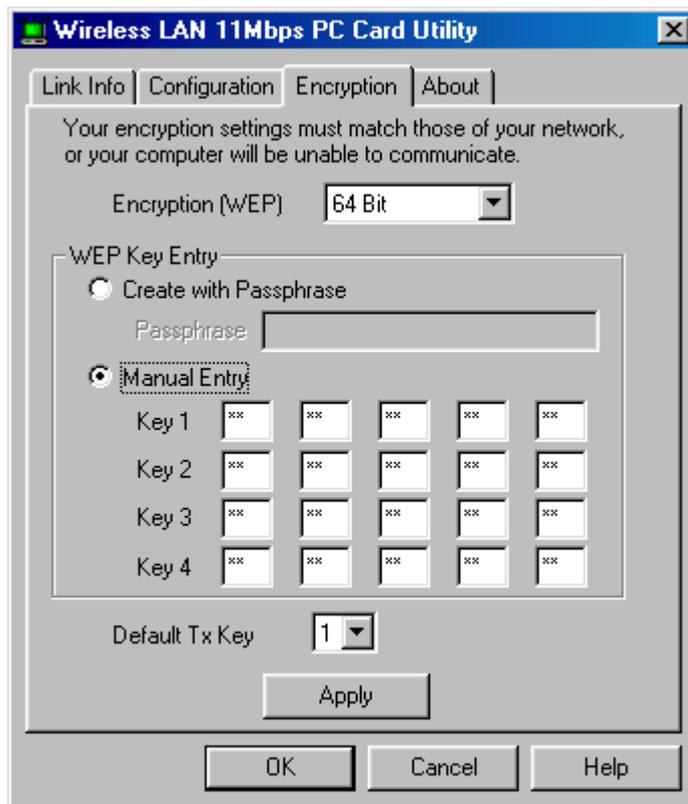
Figure 5 Management window with “Encryption” tab open
