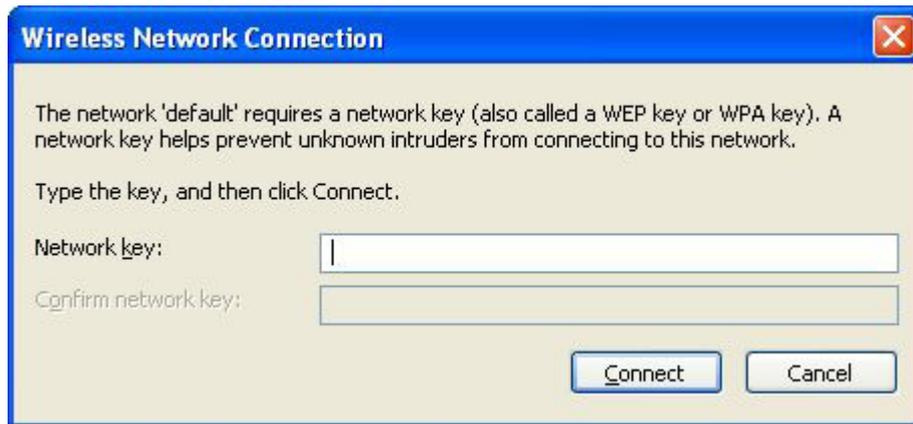
Figure 2-15 setting for security key or passphrase
