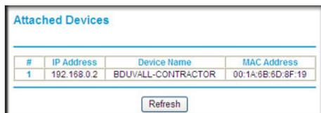
For each device, the table shows the IP address, device name if available, and the Ethernet MAC address. If the router is rebooted, this data is lost until the router rediscovers the devices. To force the router to look for attached devices, click the **Refresh** button.
