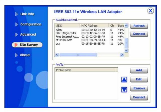
**Available Network** – displays the wireless networks (wireless clients and access points) that are within range.
