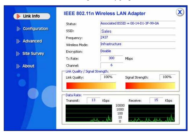
**Status:** Shows the associated BSSID, which can be used to identify the wireless access point.
