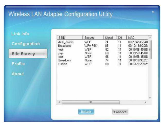
**Available Network** – displays the wireless networks (wireless clients and access points) that are within range.
