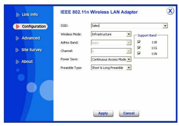
**SSID:** Service Set Identifier, which is a unique name shared among all clients in a wireless network. The SSID must be identical for each client in the wireless network.
