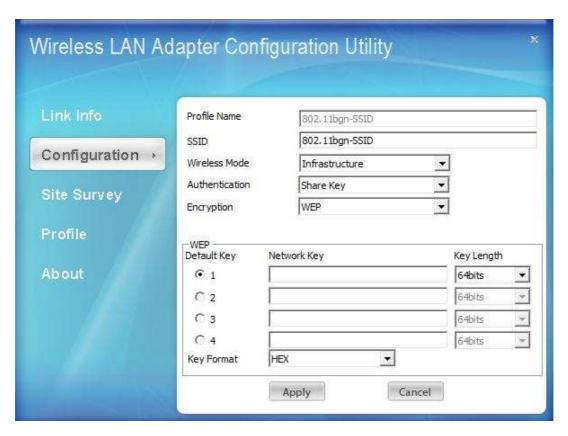
**SSID:** Service Set Identifier, which is a unique name shared among all clients in a wireless network. The SSID must be identical for each client in the wireless network.
