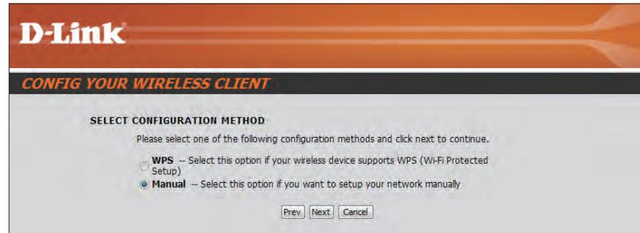
The screenshot shows the 'CONFIG YOUR WIRELESS CLIENT' screen with the 'SELECT CONFIGURATION METHOD' section. It includes instructions to select a method and two radio button options: 'WPS Setup' and 'Manual'. The 'Manual' option is selected. Navigation buttons 'Prev', 'Next', and 'Cancel' are at the bottom.
