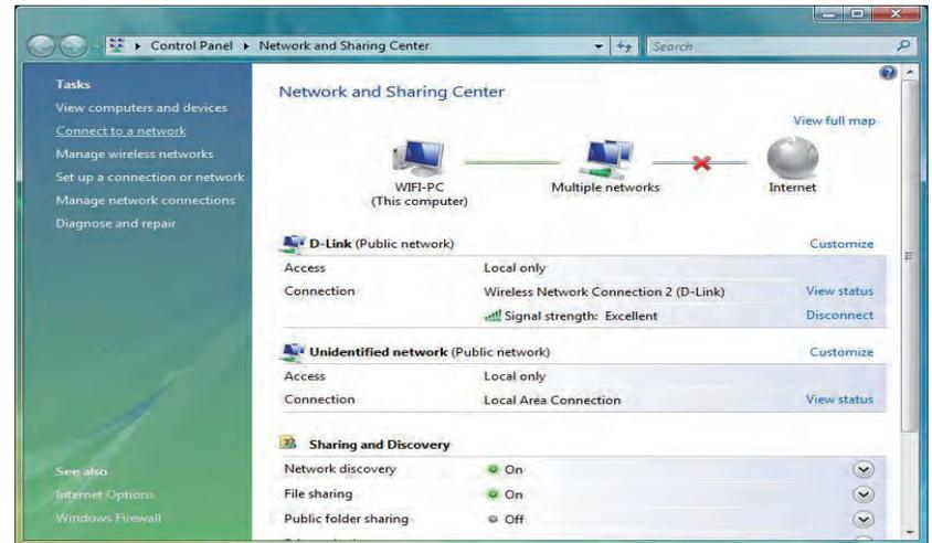
The utility will display any available wireless networks in your area. Click on a network (displayed using the SSID) under Select a network to connect to and then click the **Connect** button.
