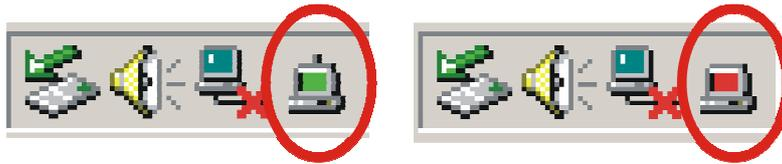
When the icon in the toolbar represents in green color, it is properly connected to the network and if it represents in red color, then it is not connected to the network.
