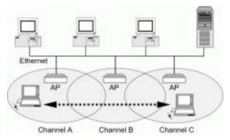
Figure 1-3 Roaming Across Multiple Access Points
