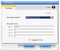
The *Encryption Method* drop down list allows you to select the type of encryption for the network. The correct encryption type should already be selected automatically.
