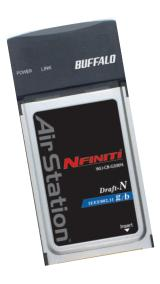
• The WLI-CB-G300N has three internal diversity antennas. External antennas can not be attached to the WLI-CB-G300N.
