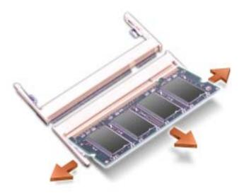
NOTICE: If you need to install memory modules in two connectors, install a memory module in the connector labeled "SLOT 1" before you install a module in the other connector.
