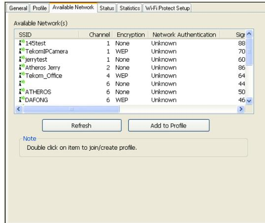
Select one of SSIDs, and click **Add to Profile** to create profile that can be configured more wireless parameters.
