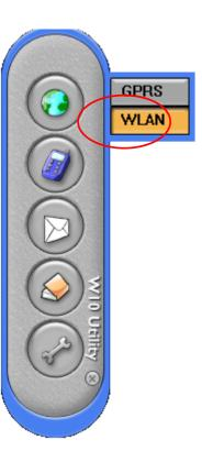
When users choose network configuration, the submenu will pop up. Left click the mouse on the WLAN item and the WLAN control panel will pop up.
