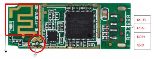
Built-in antenna test point
