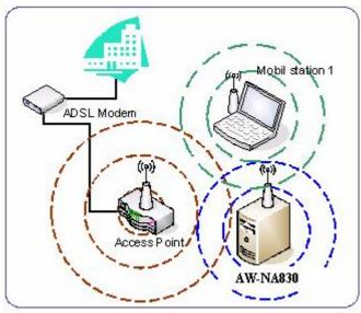
A wireless LAN enabled computer can physically move from the operating range of one access point to another without losing connection to the LAN. A quick association "hand-shake" is made between the new access point and the wireless device as the computer traverses from the coverage of one access point to another. The access point enable a wireless LAN computer to move through a building and still be connected to the LAN.
