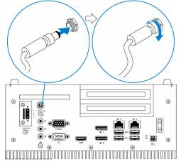
Connect the power terminal block to the adapter port and torque the screws at 5.07 kilograms-centimeter (4.4 pounds-inch) to secure it to the Embedded Box PC.
