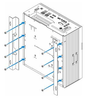
2 Drill four holes in the wall that correspond to the holes on the mounting bracket.
