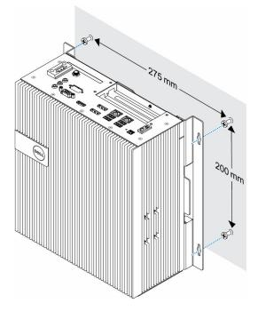
Secure the Embedded Box PC to the wall. 4
