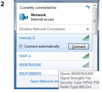
Select the target AirStation's name and click [Connect]. If you will be connecting to this device in the future, checking [Connect automatically] is recommended.
