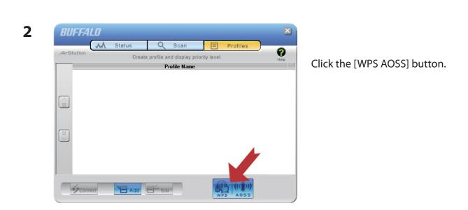
Follow any instructions displayed on the screen. When the Security LED on the front of the AirStation stops flashing and is lit steadily, the connection is complete.
