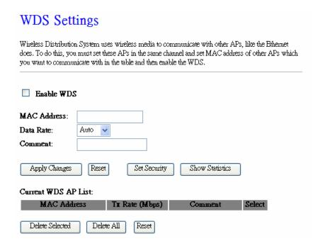
**Step 1.** Check the MAC address and Channel number of the device you want to setup WDS with 11N Broadband Router.
