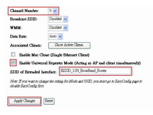
Note: The DHCP server should be disabled under menu "LAN Interface Setup" and then the URM could be enabled.
