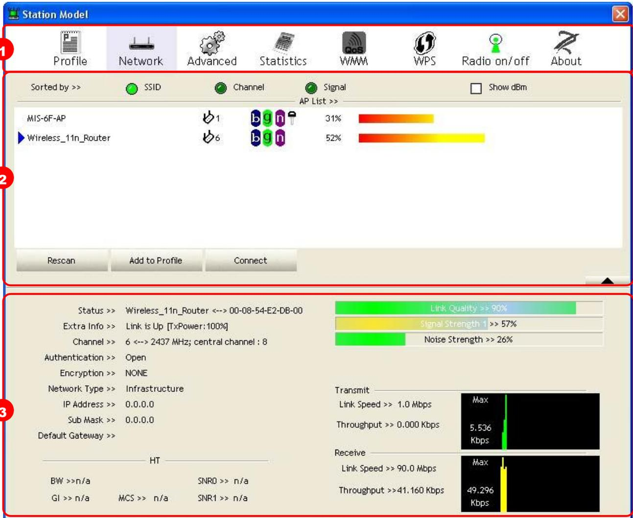
**1. Functional Buttons:** on top of the window. You can click each button to access each configuration window.
