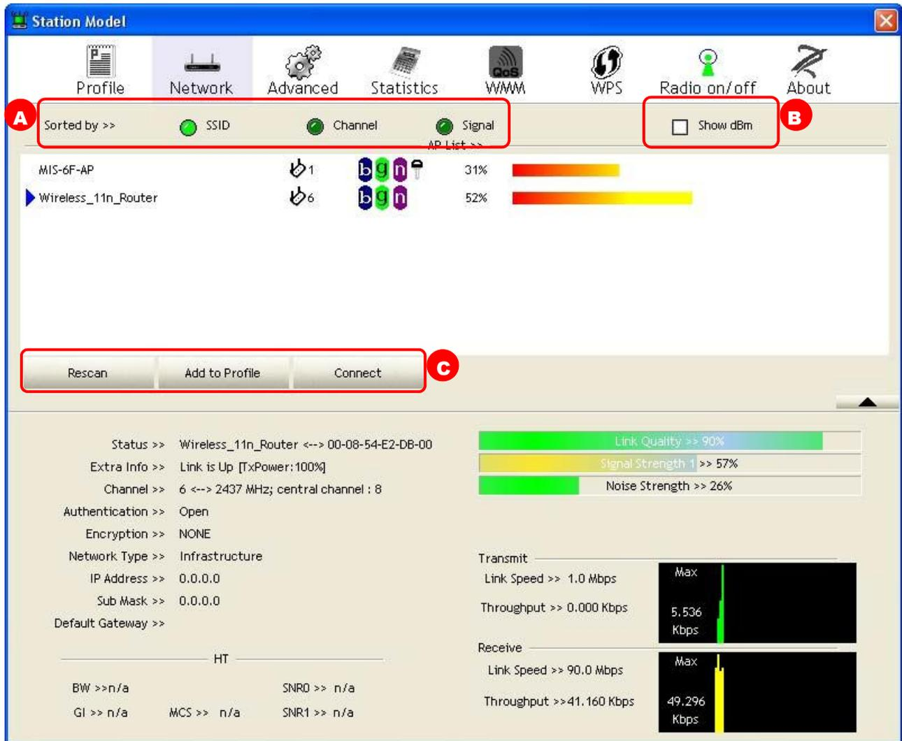
**A. Sorted by:** Click each button to sort the listing networks by SSID, channel and Signal strength.
