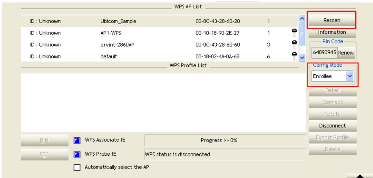
3. Select an AP (SSID/BSSID) that STA will join to.
