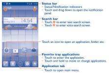
Home screen is provided in an extended format to allow more space for adding applications, shortcuts etc. Slide the Home screen horizontally left and right to get a complete view of the Home screen. Blue line at the lower left and right of the screen indicate which screen you are viewing. You can customize the number of home screens by **Settings\Display\ Home screen settings**.
