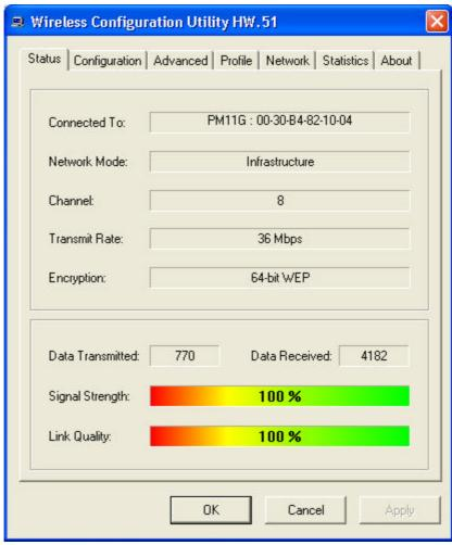
There is another dialog box showing the data transmitted and data received. The two signal lines show the Signal Strength and the Link Quality of the device.
