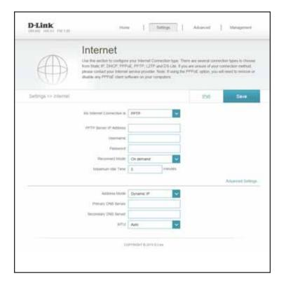
**Secondary DNS** Enter the secondary DNS server IP address assigned by your ISP. **Server:**
