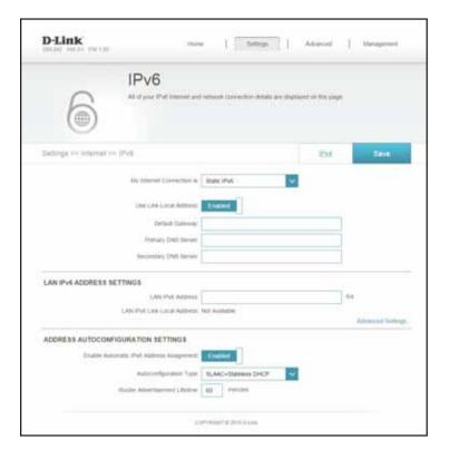
**Autoconfiguration** Select Stateful (DHCPv6), SLAAC + RDNSS or SLAAC + Stateless **Type:** DHCPv6.
