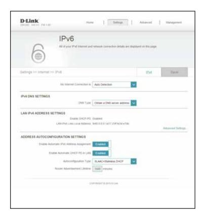
**Autoconfiguration** Select Stateful (DHCPv6), SLAAC + RDNSS or SLAAC + Stateless **Type:** DHCPv6.
