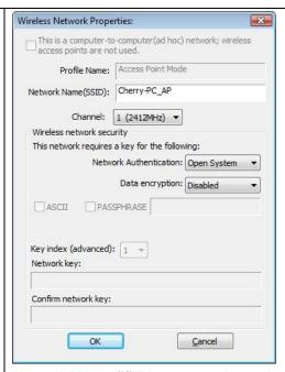
**Network Name (SSID):** User can change the network name of this access point.
