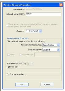
**Network Name (SSID):** User can change the network name of this access point.
