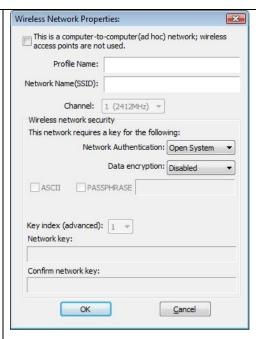
This is a computer-to-computer (ad hoc) network; wireless access points are not used: This function is selected to enable the ad hoc network type that computers should be setup at the same channel to communicate to each other directly without access point, users can share files and printers between each PC and laptop.
