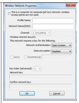
This is a computer-to-computer (ad hoc) network; wireless access points are not used: This function is selected to enable the ad hoc network type that computers should be setup at the same channel to communicate to each other directly without access point, users can share files and printers between each PC and laptop.
