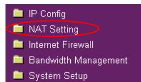
2. Select **Yes** to enable virtual server. For example, if host 192.168.1.100 is the FTP server that the user will access, it means all packets from Internet with destination port as 21 are to be directed to the host. Set Well-known Application to FTP. Port range to 21, Local IP to the host IP, Local Port to 21, Protocol to TCP.
