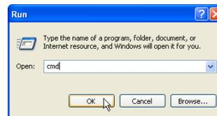
18. Type **ping account.dyndns.org** (your DDNS domain name). If you can see the reply like what is shown in the right picture, DDNS is working correctly.
