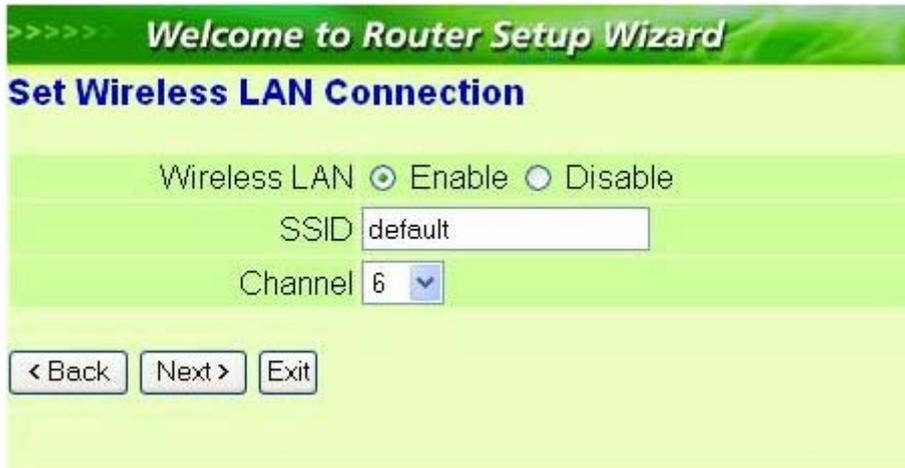
The screenshot shows the 'Set Wireless LAN Connection' screen of the Router Setup Wizard. At the top, it says 'Welcome to Router Setup Wizard'. Below that, the title is 'Set Wireless LAN Connection'. There are three rows of settings: 'Wireless LAN' with radio buttons for 'Enable' (selected) and 'Disable'; 'SSID' with a text box containing 'default'; and 'Channel' with a dropdown menu showing '6'. At the bottom, there are three buttons: '< Back', 'Next >', and 'Exit'.
