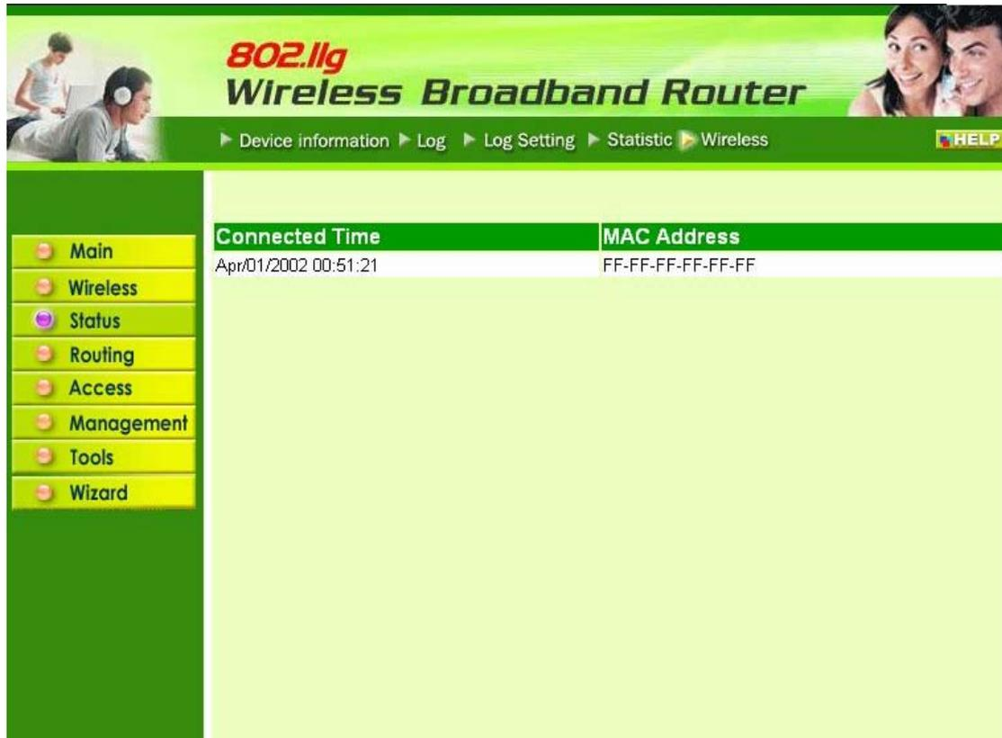
**Connected Time:** Displays how long the wireless device has been connected to the LAN via the router.
