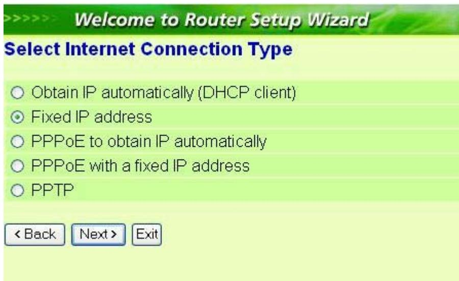
If the Internet Service Providers assign a fixed IP address, choose this option and enter the assigned IP address, subnet mask, gateway IP and DNS IP addresses for your Broadband Router.
