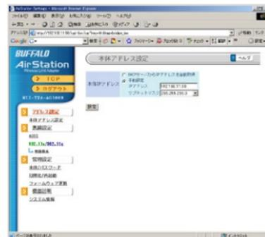
This is the advanced page. On the left, you may choose from Wireless Settings, Network Settings, or Management. When the page first opens, it's at Wireless Settings. Changes on advanced pages are not applied until the *Apply* button is pressed.
