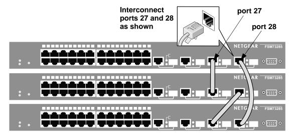
Figure 12-1: Interconnecting individual FSM7328S switches to form a stack
