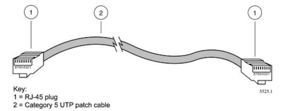
Figure 12-5: Category 5 UTP Cable with Male RJ-45 Plug at Each End
