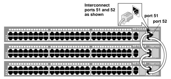
Figure 12-2: Interconnecting individual FSM7352S switches to form a stack
