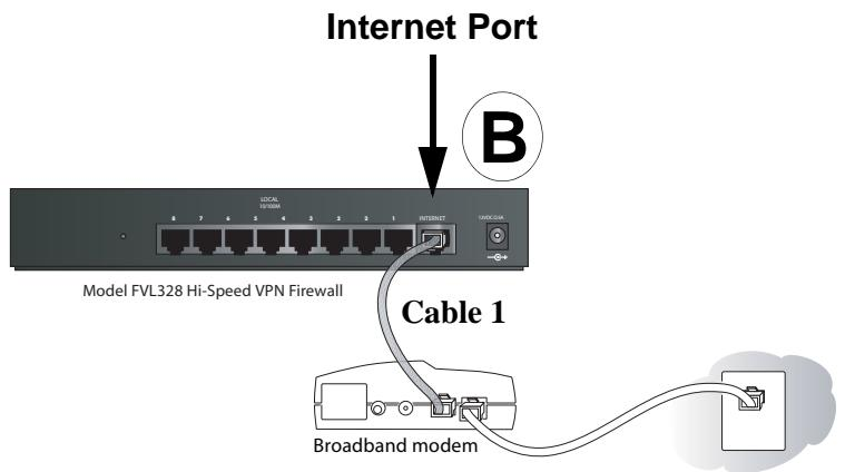
**Figure 3-2: Connect the broadband modem to the router**
