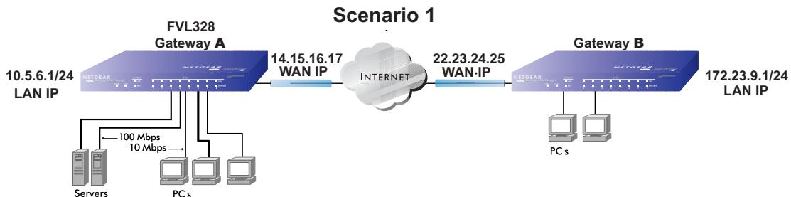
Figure 6-11: LAN to LAN VPN access from an FVL328 to an FVL328
