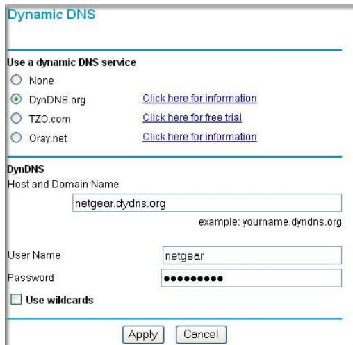
Figure H-2: Dynamic DNS Setup menu
