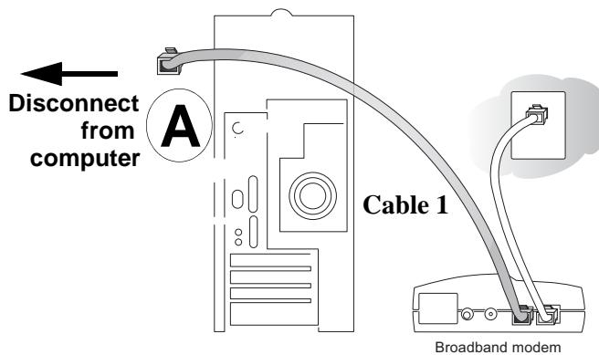
**Figure 3-1: Disconnect the broadband modem**
