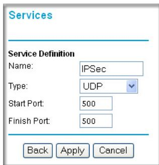
**Figure 5-5: Service example: port forwarding for VPN when NAT is Off**
