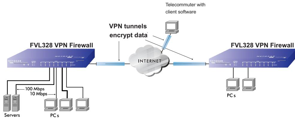
Figure 6-1: Secure access through FVL328 VPN routers
