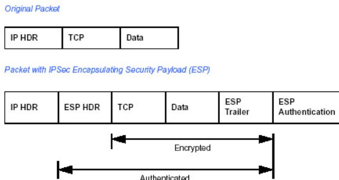
**Figure E-1: Original packet and packet with IPSec Encapsulated Security Payload**
