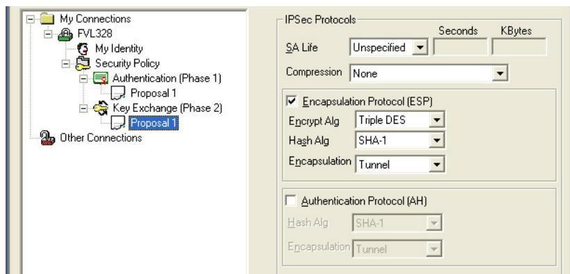
**Figure G-11: Connection Security Policy Key Exchange (Phase 2)**
