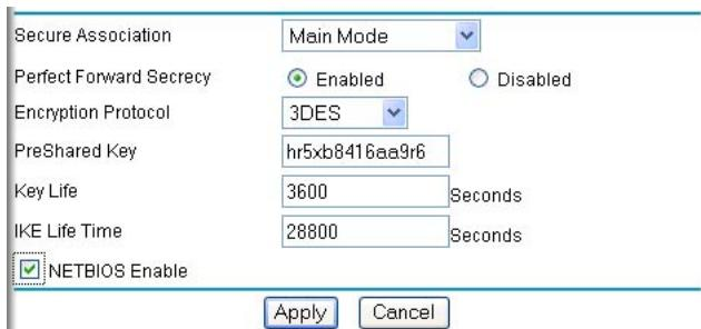
**Figure H-5: Figure 4 – NETGEAR FVS318 VPN Settings (part 2) – Main Mode**
