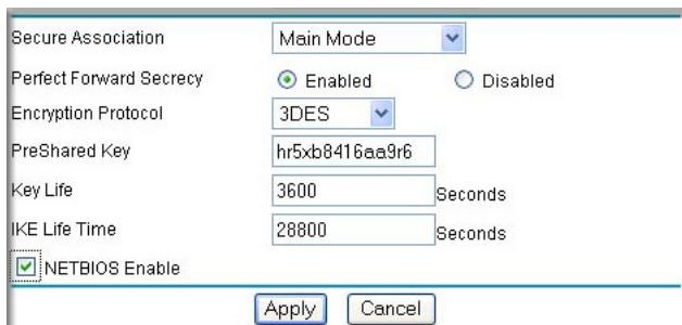
**Figure F-4: Figure 4 – NETGEAR FVS318 VPN Settings (part 2) – Main Mode**
