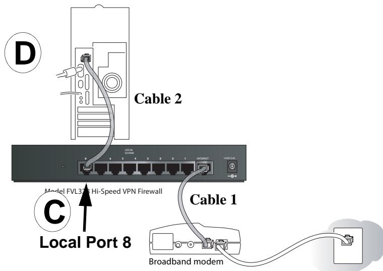
**Figure 3-3: Connect the computers on your network to the router**
