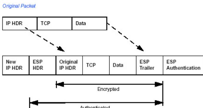
**Figure E-3: Original packet and packet with IPSec ESP in Tunnel mode**
