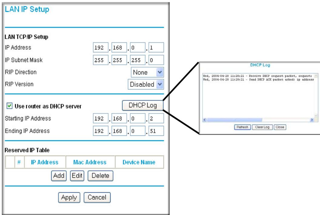
**Figure 4-1: LAN IP Setup Menu**
