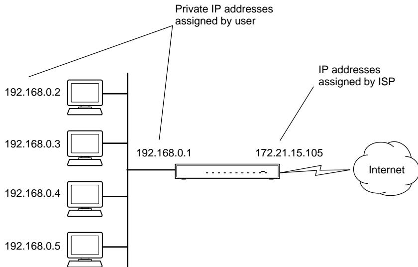
**Figure 8-3: Single IP Address Operation Using NAT**
