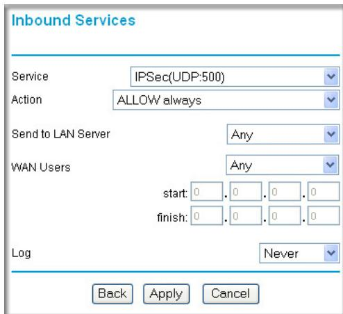
**Figure 5-6: Inbound rule example: VPN IPSec when NAT is off**
