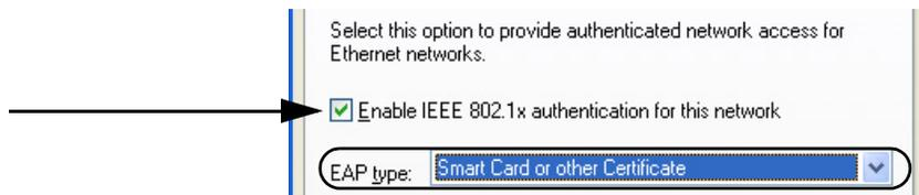
**Figure 5-4: Configure a Windows XP wireless adapter for EAP-TLS**
