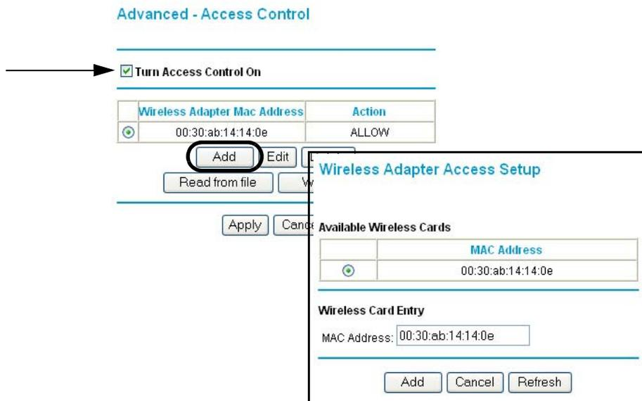
**Figure 3-10: Wireless Card Access List Setup**
