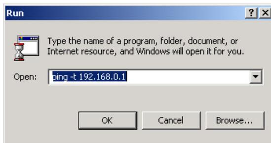
Figure 5-6: Running a Ping test from Windows
