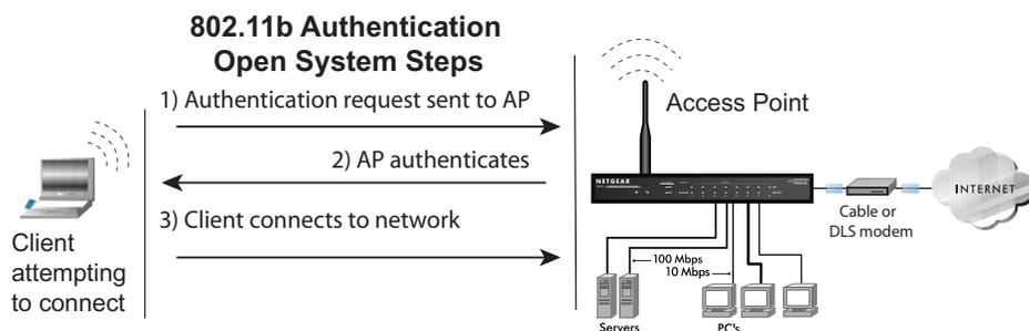
**Figure 6-1: 802.11 open system authentication**
