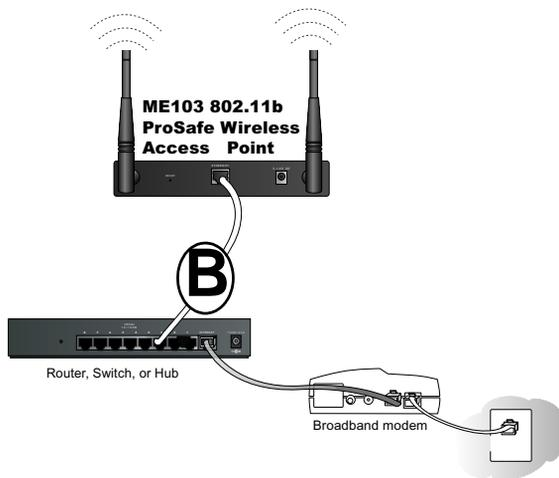
**Figure 3-3: Connecting the Ethernet cable to a router, hub, or switch**
