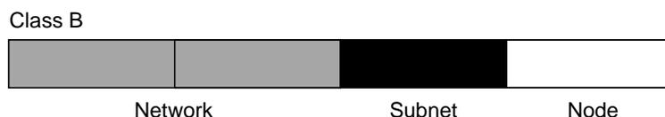
**Figure B-2: Example of Subnetting a Class B Address**
