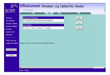
Check the *Enable SPI and Anti-Dos* Firewall protection check box to enable SPI. When this feature is enabled, all incoming packets will be blocked except for those types that you allow in the Stateful Packet Inspection section.
