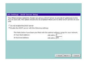
To activate the DHCP Server option, select *Enable the DHCP server with the following settings:* and specify the IP pool range. The largest available continuous IP pool will be automatically entered; if this is not appropriate, make your required changes. To disable DHCP, select *Do not enable the DHCP server*. Click *Next* when you have finished.
