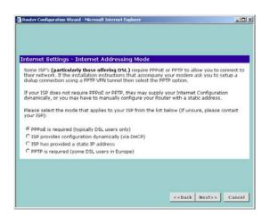
This *Internet Addressing Mode* window allows you to set up the Router for the type of Internet connection you have. Before setting up your
