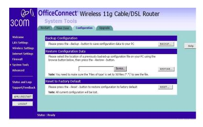
Select the Configuration tab to display the Configuration screen .
