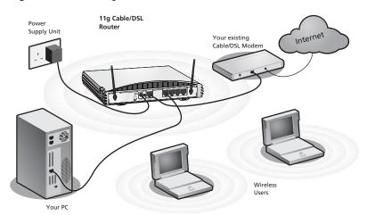
**Figure 5** Connecting the Router
