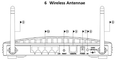
The antennae on the product should be placed in a 'V' position when initially installed.
