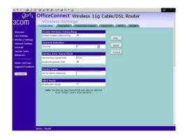
This screen displays the Channel and Service Area Name. It also allows you to change these settings. There are a maximum of 14 channels, the number available to you is dependent on the country you reside in. Selecting *Clear Channel Select* from the *Channel* drop-down list allows the Router to automatically select an available channel when first powered on.
