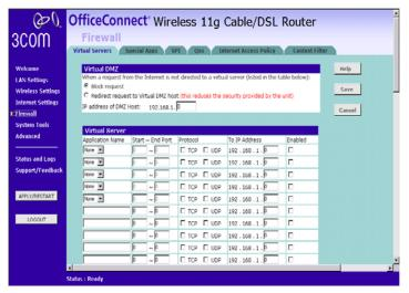
**Virtual DMZ** DMZ (De-Militarized Zone) Host is a computer without the protection of the firewall. This feature allows a single computer to be exposed to unrestricted 2-way communication from outside of your network. This feature should be used only if the Virtual Server or Special Applications options do not provide the level of access needed for certain applications.
