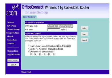
Figure 35 Connection Parameters Screen - Dynamic IP
