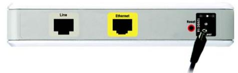
Figure 4-3: Connect the Power
