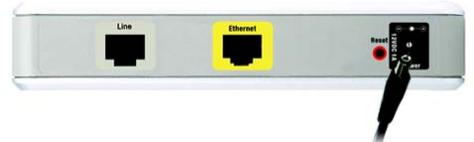
Figure 4-5: Connect the Power
