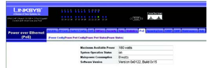
Figure 5-58: PoE - Power Status
