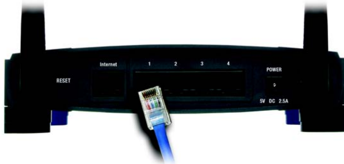
Figure 4-2: Connecting Your Network Devices
