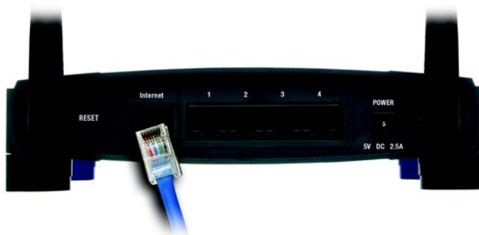
Figure 4-5: Connecting Another Router
