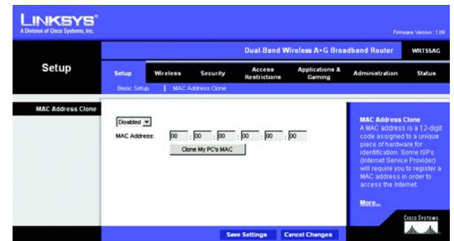
Figure E-5: MAC Address Clone
