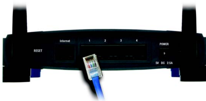
Figure 4-6: Connecting Your Network Devices
