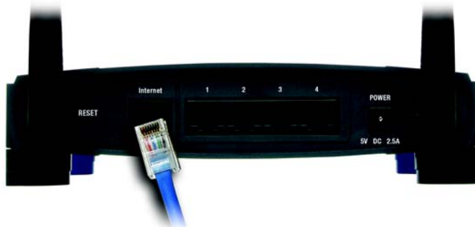
Figure 4-1: Connecting Your Broadband Modem
