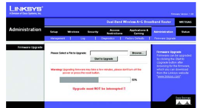
Figure 5-32: Administration Tab - Firmware Upgrade
