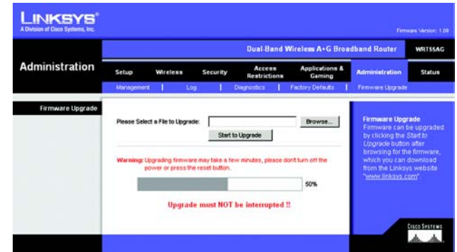
Figure C-1: Administration Tab - Firmware Upgrade
