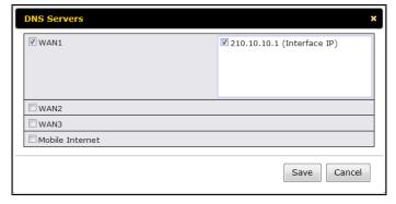
To specify the Internet IP addresses on which the DNS Server should listen, select the desired WAN connection then select the desired associated IP addresses. (Multiple items in the list can be selected by holding CTRL and clicking on the items.)
