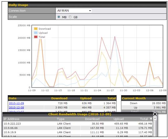
Click on a specific date to receive a breakdown of all client usage for that date.
