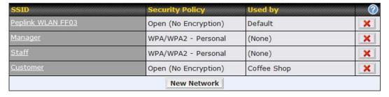
Click the button **New Network** to create a new Network profile, or click the existing network profile to modify its settings.
