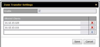
The Peplink Balance serves both the clients that are accessing from the specified IP addresses, and the clients that are accessing its LAN Interface.
