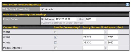
When this feature is enabled, the Peplink Balance will intercept all outgoing connections destined for the proxy server specified in "Web Proxy Server Interception Settings". Then it will choose a WAN connection according to the Outbound Policy and forward the connection to the specified web proxy server and port
