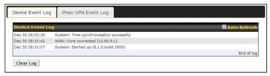
The log section displays a list of events that has taken place on the Peplink Balance unit. Click the **Refresh** button to retrieve log entries again. Click the **Clear Log** button to clear the log. Select **50**, **100**, or **all** to show the corresponding number of events in the log.
