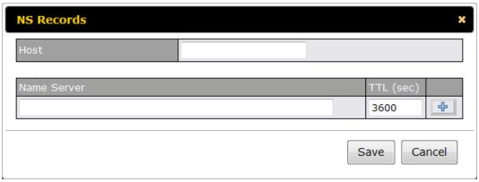
The NS record of the name server defined in the SOA record is automatically added here. To create a new NS record, click the **New NS Records** button.
