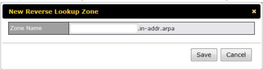
Reverse lookup refers to performing a DNS query to find one or more DNS names associated with a given IP address.
