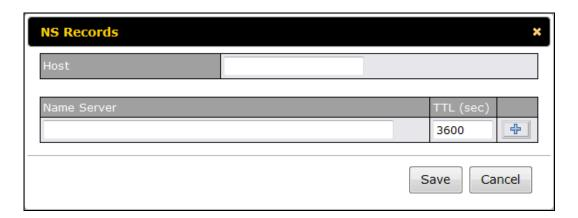
When creating an NS record for the domain itself (not a sub-domain), the **Host** field should be left blank. Enter a name server host name and its IP address into the corresponding boxes. The host name can be a non-FQDN (fully qualified domain name) (please be sure that a corresponding A record is created). Click the button on the right to finish and to add other Name Servers.
