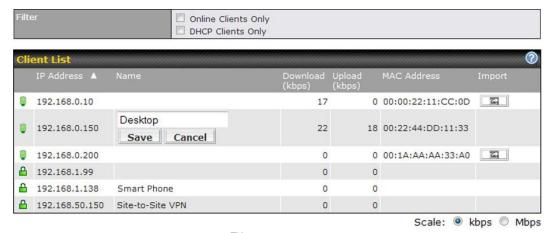
If PPTP Server in section **22.2**, SpeedFusion<sup>TM</sup> in section **12.1**, or AP Controller in section **18** is enabled, you may see the corresponding connection name listed in the **Name** field.
