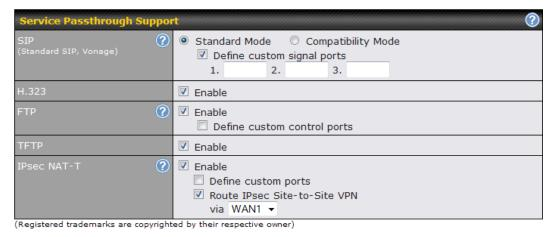
Some Internet services need to be specially handled in a multi-WAN environment. The Peplink Balance can handle these services such that Internet applications do not notice it is behind a multi-WAN router. Settings for Service Passthrough Support are available here.
