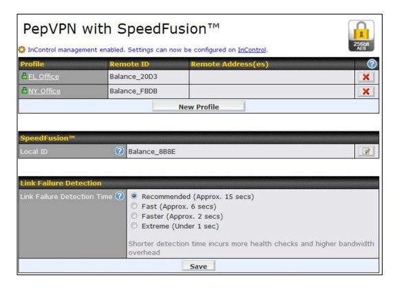
To configure a new SpeedFusion<sup>™</sup> profile, navigate to **Network>SpeedFusion**<sup>™</sup>>**New Profile**
