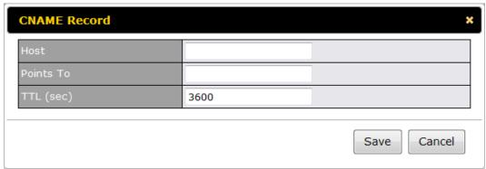
When creating a CNAME record for the domain itself (not a sub-domain), the Host field should be left blank.
