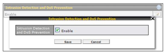
The Balance can detect and prevent intrusions and Denial-of-Service (DoS) attacks from the Internet. To turn on this feature, click , check the **Enable** check box for the **Intrusion Detection and DoS Prevention** and press the **Save** button.
