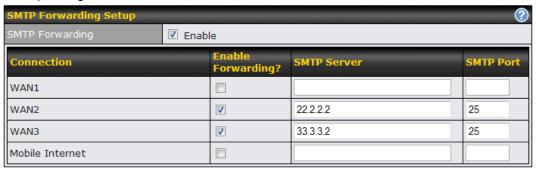
To enable the feature, select the *Enable* check box under **SMTP Forwarding Setup**. Check the box *Enable Forwarding* for the WAN connection(s) that needs such forwarding. Under **SMTP Server**, enter the ISP's e-mail server host name or IP address and under **SMTP Port**, enter the TCP port number for each WAN.
