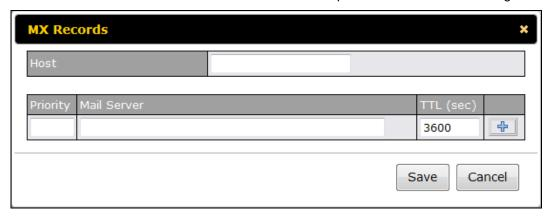
When creating an MX record for the domain itself (not a sub-domain), the **Host** field should be left blank. For each record, **Priority** and **Mail Server** name must be entered. **Priority** typically ranges from 10 to 100. Smaller numbers have a higher a priority.
