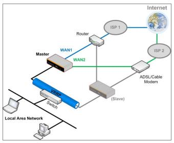
In the diagram, the WAN ports of each Peplink Balance unit connect to the router and to the modem. Both Peplink Balance units connect to the same LAN switch via a LAN port.
