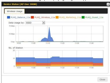
Click any point in the graphs to display detailed usage and client information for that device, using that SSID, at that point in time. On the **Data Usage by** menu, you could choose to display the information by SSID or by AP Send/Receive rate.
