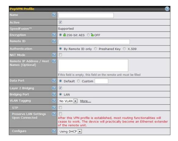
A list of defined SpeedFusion<sup>TM</sup> connection profiles and a **Link Failure Detection Time** option will be shown. Click the **New Profile** button to create a new VPN connection profile for making a VPN connection to a remote Peplink Balance via the available WAN connections. Each profile is for making a VPN connection with one remote Peplink Balance.
