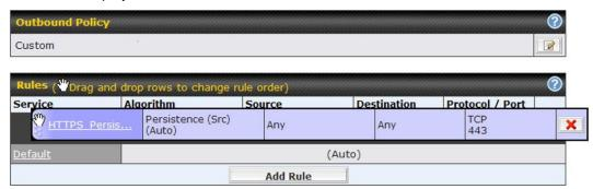
The bottom-most rule is **Default**. Edit this rule to change the device's default manner of controlling outbound traffic for all connections that do not match any of the rules above it. Under the **Service** heading, **Default** to change these settings. To rearrange the priority of outbound rules, drag and drop them into the desired sequence.
