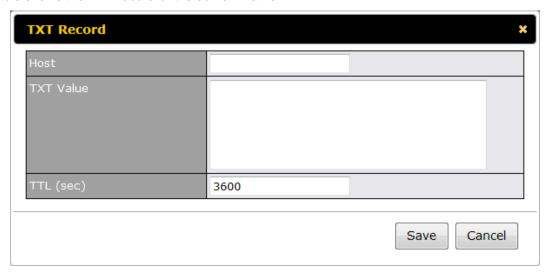
To add a new TXT record, click the **New TXT Record** button in the **TXT Records** box. Click the **Edit** button to edit the record. The time-to-live value and the TXT record's value can be entered. Click the **Save** button to finish.
