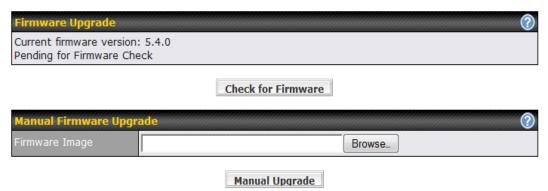
There are two ways to upgrade the unit. The first method is through an online download, the system can **Download and Upgrade** over the Internet. The second method is to upload a firmware file manually.
