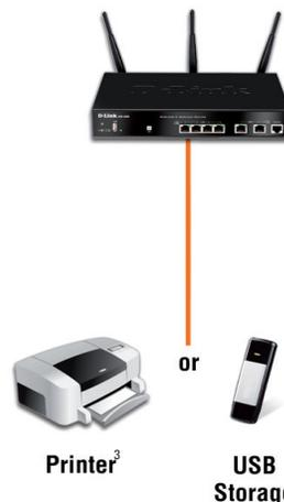
Supports one (DSR-250N/500N) or two (DSR-1000N) USB 2.0 devices to extend functionality via D-Link's SharePort feature.
