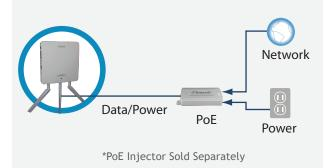
By combining your power and data connections into a single cable, PoE can simplify the setup. This gives you flexibility to install the device in any location, even out of the way locations with few power outlets.
